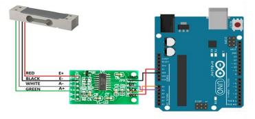
Figure 5: Hardware organization of Weight Sensor
