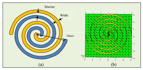
Figure 1: Basic structure of a linear spiral antenna
