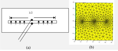
**Figure 2:** A  $\lambda/2$  slot antenna
