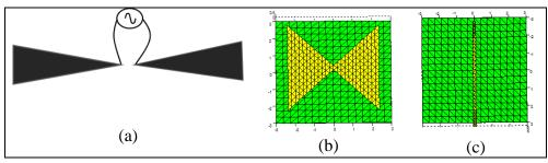
Figure 3: Bowtie and dipole antennas
