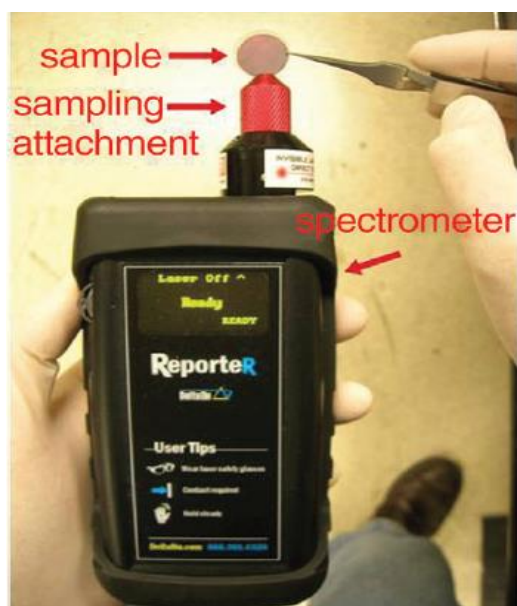
Figure 4: A palm-size SERS device capable of screening samples in the field level ( Sharma et al., 2012 ).
